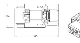
\*) 39.1mm (condition of delivery | 35.1mm (Second locking activated)
